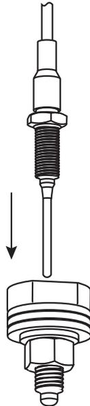
Screw the M8 threaded part of the probe into the probe housing until it can go no further then tighten the M8 locknut to stop it vibrating loose.
