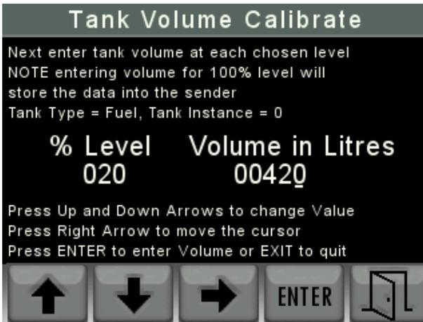
The user then enters the volume of fluid at each desired level starting at the lowest chosen point in as many or as few steps to 100%.
