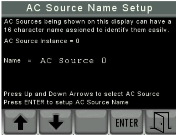
Firstly, by pressing the up arrow and down arrow buttons select the AC Source instance to be named then press “ENTER”.
