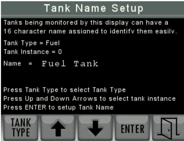
Firstly the user must select the tank type that is being named by pressing the "TANK TYPE" button. This will cycle around all the available tank types and the display must be left on the type of tank to be named.
