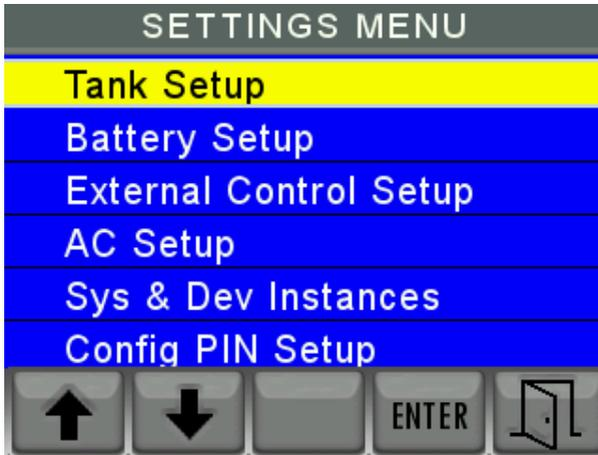
Note the small arrow on the left hand screen indicates that there are more options than can be shown on one page. All these options and the ones not shown are accessed by moving the yellow highlighter to the chosen option and then pressing “ENTER”
