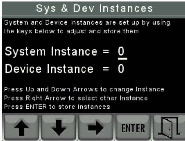
The user should use the “UP” and “DOWN” arrows to change the value of the Instance that is underlined and then use the “RIGHT” arrow to select the other Instance.
