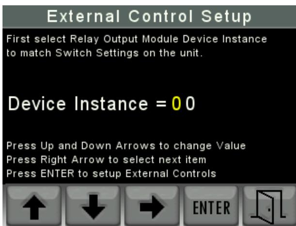
When the Device Instance has been chosen pressing “ENTER” will go to the next screen to allow choice of the actions to operate each of the eight relays in the 3478 unit.
