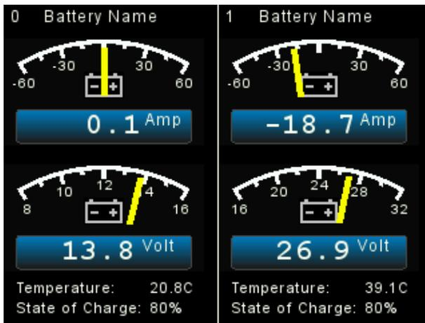
Repeated pressing of the “BATT” button will display the next two batteries or DC sources to a total of 16 sources. Each side of the display contains the following information:
