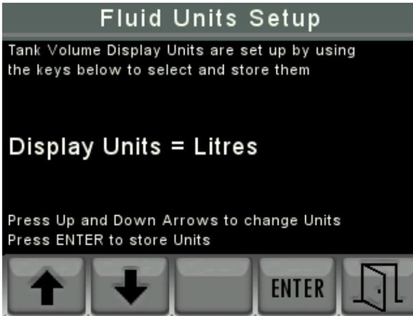
The user can change the units by using the “UP” and “DOWN” arrows and pressing “ENTER” to select their units of choice. Pressing “EXIT” will return to the “SETTINGS MENU”
