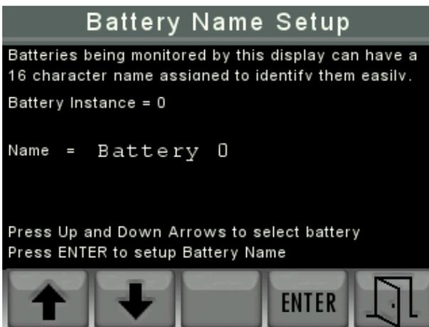
Firstly, by pressing the up arrow and down arrow buttons select the battery instance or battery number to be named then press “ENTER”.
