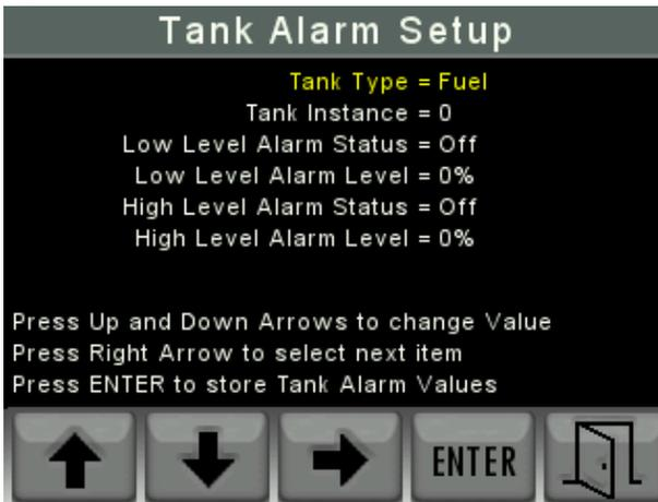
The user can select both low and high level alarms for each tank and the alarm level for each type of alarm.
