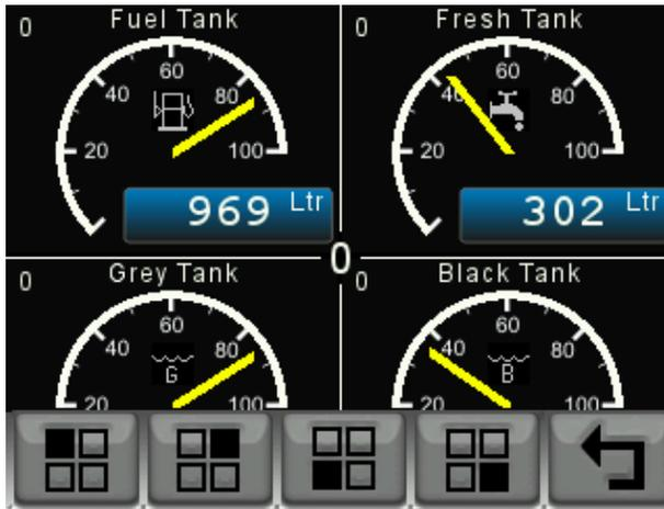
Pressing the first button the top left hand quadrant will change to display each of the different tank sender levels being received and then a blank page in case the user does not wish to display any tank in a given quadrant. Then by pressing the “BACK ARROW” button selection will be remembered and the display will revert to the normal tank display. This can be repeated for each quadrant on each Quadrant Page giving the user the opportunity to tailor the tank displays exactly as they wish.
