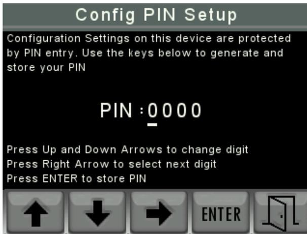
The user can use the “UP” and “DOWN” arrows to change the value of the underlined PIN number and then use the “RIGHT” arrow to choose the next number to change. When the desired PIN number has been chosen pressing the “ENTER” key will store it and then pressing the “EXIT” key will return to the settings menu.
