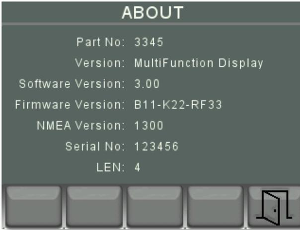
This screen displays data about the unit including the software version and unit serial number which will identify the exact unit if requested.
