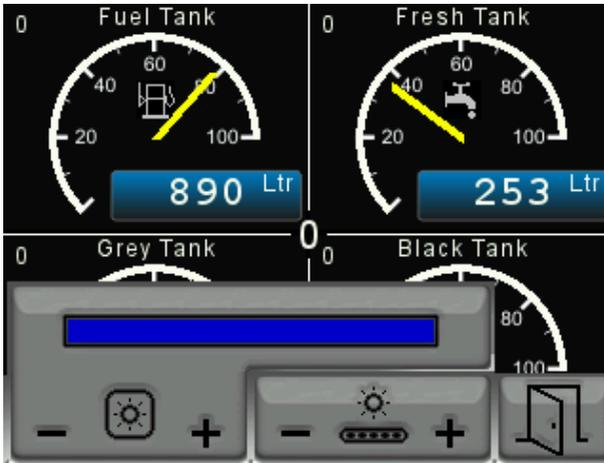
Pressing the first two buttons varies the screen brightness and the next two buttons vary the key backlights. When the desired levels have been set press the fifth button to clear the display brightness control.
