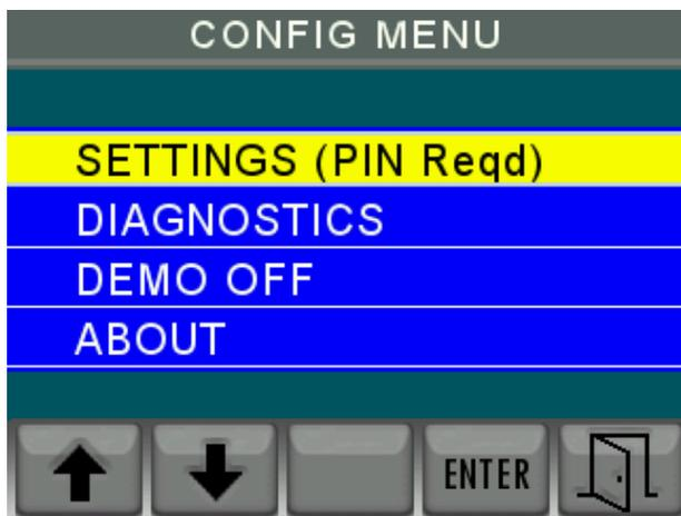
On this menu use the up and down arrow keys to change the yellow highlight to the action required and then press “ENTER”
