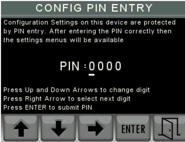
By using the Up and Down and Right arrow buttons the user selected PIN can be entered and the “ENTER” key will go to the “SETTINGS MENU” if the PIN is correct. If the PIN is not correct the user is offered the choice to re-enter the PIN or exit back to the “CONFIG MENU” detailed in 3.1 above.
