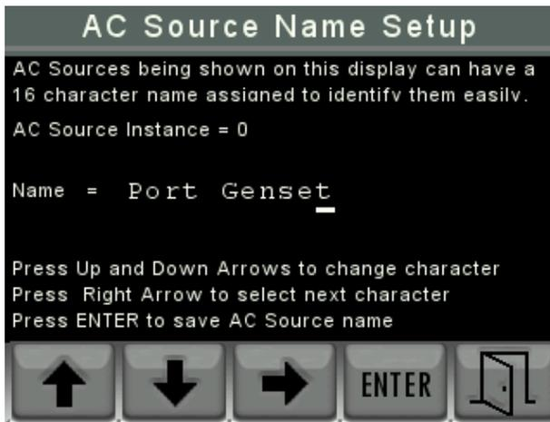
Next use the Up and down arrow keys to change the first character of the name then press the right key to move to be able to change the next character and so on. Please note that the characters will cycle through A to Z upper case then a to z lower case, then a blank then numbers from 0 to 9.
