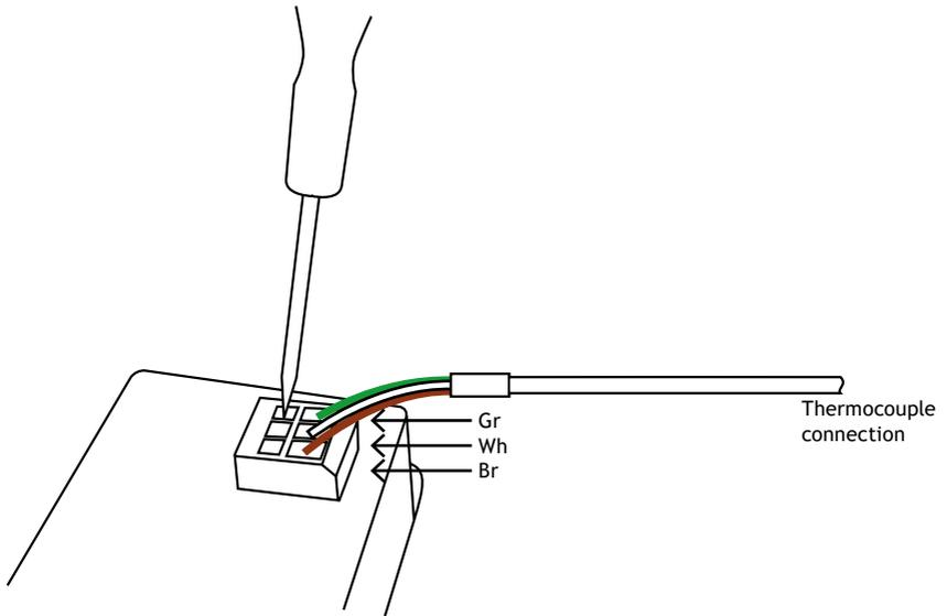
Check that the cage clamp is making contact with the bared wire end and is not seated onto the wire insulation.
